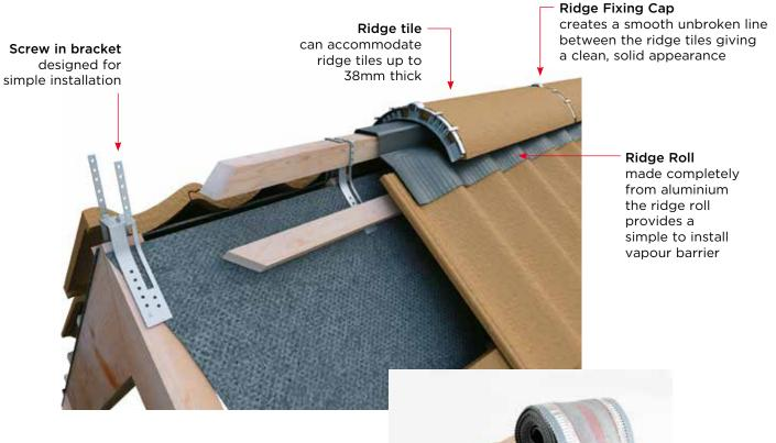
The Corovent dry fix system is supplied as a complete system with all the components to fix 6m of ridge.
