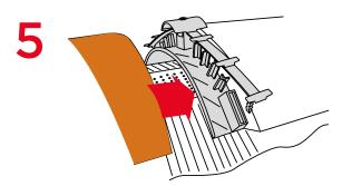
Push next ridge tile firmly into place, trapping it between the cap and union (see note 'b' below)
